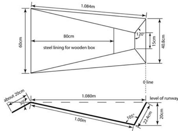
Figure 7 - Pole vault box (top and side view)
