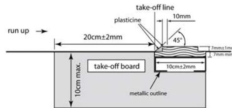
Figure 10 - Take-off board and plasticine indicator board
