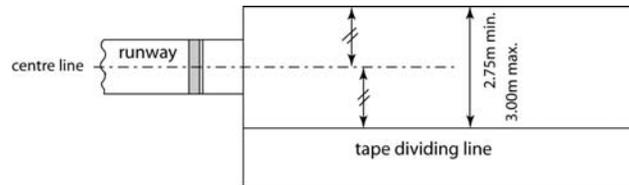
Figure 11 - Centralised Long Jump / Triple Jump landing area
