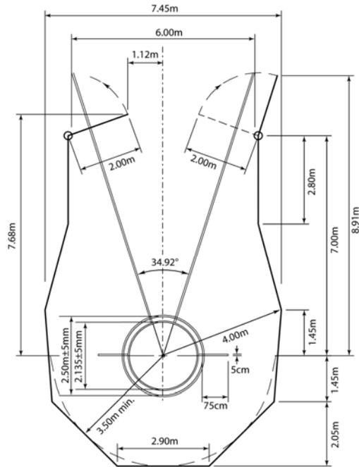
Figure 22 - Cage for Hammer and Discus Throw with concentric circles
